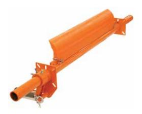
The Martin<sup>®</sup> QC1<sup>™</sup> Cleaner PD provides maximum durability and performance across a wide range of duties and applications. This sturdy cleaner features one-pin blade change, making replacement of a worn blade a simple procedure. The one-piece urethane blade has a "CARP" (Constant Angle Radial Pressure) design to maintain cleaning performance through all stages of blade life.
